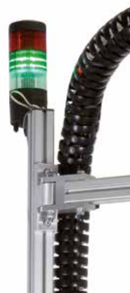
Signal lamps indicate the operating status
